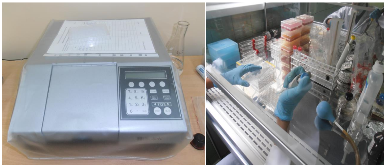
Fig. 14 Multiwell spectrophotometer ("reader") for automatic determination of colorimetric/spectrophotometric indicators in 96-well tablets. Addition of MTT to 96-well plates and staining after dissolution of formazan crystals
