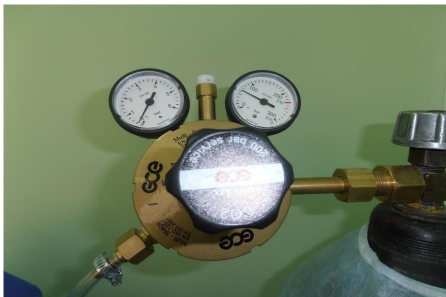
Fig.2.Reducer to carbon dioxide cylinder
